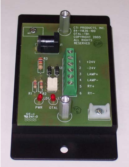
Figure 3 Board & Spacers Installed
